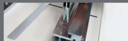
Remove the hole punch by tweezers. Ensure you put the hole punches that are removed back in the same place.
