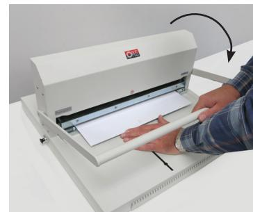
1. Move the handle to the open position. Remove previous module. Insert the 0.Punch / Closer MP 52 46/3: 1 + thumb cut or 0.Punch / Closer MP 52 49/3: 1 into the slot.
