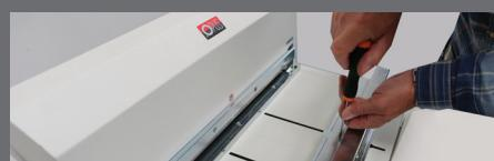
Remove the security screws and plate .
