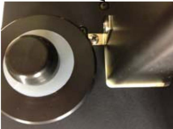
STEP (2): Remove the screw holding the bracket to the arm. NOTE:
