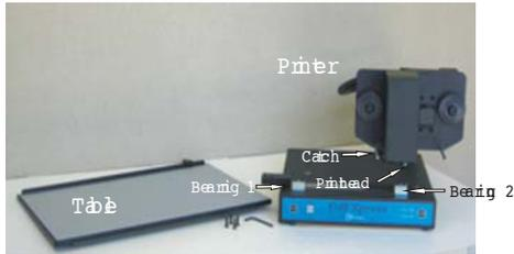
The table is attached to the printer by sliding it through Bearing 1. Continue sliding under the Catch (located at the rear of the printer) and Bearing 2 (located in the right front of the printer).
