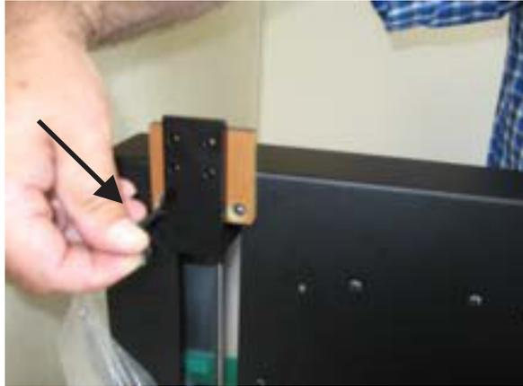
STEP (4): Remove the transportation spacer and store with other packaging materials. **NOTE: SAVE THE 4 SCREWS -- they are used to attach print bed table to main frame.**
