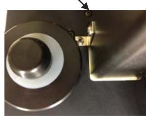
STEP(1): A medium phillipsscrew driver is needed to remove the bracket.
