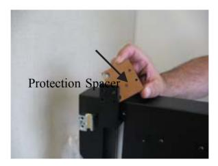
Shipping the printer without following these directions will result in damage to the printer.
