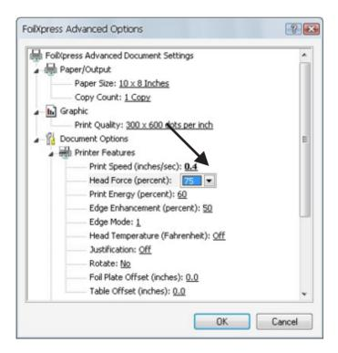
**Print Energy** The relative energy delivered to each printhead element when the element is on. This determines the temperature of the printhead elements when printing.
