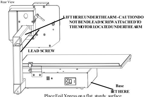
Place Foil Xpress on a flat, sturdy, surface. The unit is 20" wide x 22" deep x 13" high (51 cm x 56 cm x 33cm). Ideally, the workspace on which Foil Xpress is positioned should accommodate at least twice the weight of the printer.
