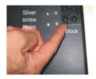
Once the table is on the printer, slide so that the right edge of the table is aligned with the right side of base of the printer (side where Bearing 2 is located).
