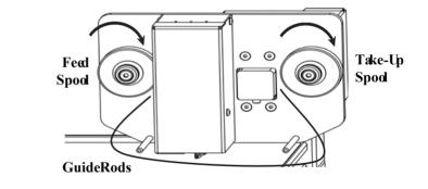
2) Slide an empty take-up core on the Take-Up Spool to collect the used film. Make certain that the metalring on the end of the tub is against the flange on the Take-Up Spool.
