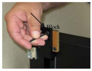
STEP (3): Remove the other two screws that attach the protection pacer to the main frame of the printer.
