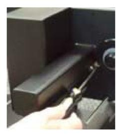
STEP (4): Make sure that you save the bracket and reattach before shipping the printer. This part and the transportation spacer bould be saved along with all of the other packaging materials.
