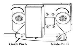
**Caution:** It is very important for the film to travel correctly. Wrinkles in the film will cause defects in printing.
