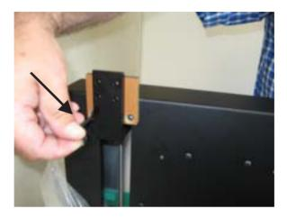
STEP (4): Remove the transportationspacer and store with other ackaging materials. NOTE: SAVE THE 4 SCREWS -they are used to attach print bed table to main frame.
