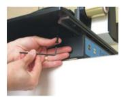
Tighten screws with the allen wrench provided.
